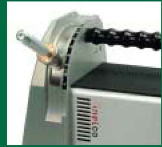
Grinding angle from 7.5 – 90° creates accurate electrode angles of 15-180°.
