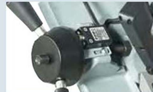
✓ Mechanical blade tension microswitch.
