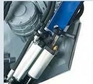
✓ Adjustable tension of the return spring to position the sawframe just above the material to be cut.
